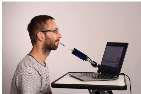
The FLipMouse module with its printed circuit board and sensors; demonstration of a possible usage scenario
