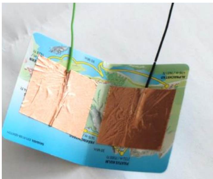
Figure 10: copper foil and the two wires stick on the inner side of the carton
