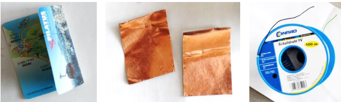
Figure 9: material for low tech switch: left picture: piece of carton, middle picture: copper foil, right picture: switch wire
